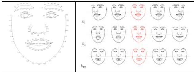
Figure 1. *Face mask model (left) and deformations of the face mask when changing one PA of the face mask b1-b17 (right). Parameter b1 changes the rotation of the head, b3 the opening of the mouth, b10 moves the pupils.*
